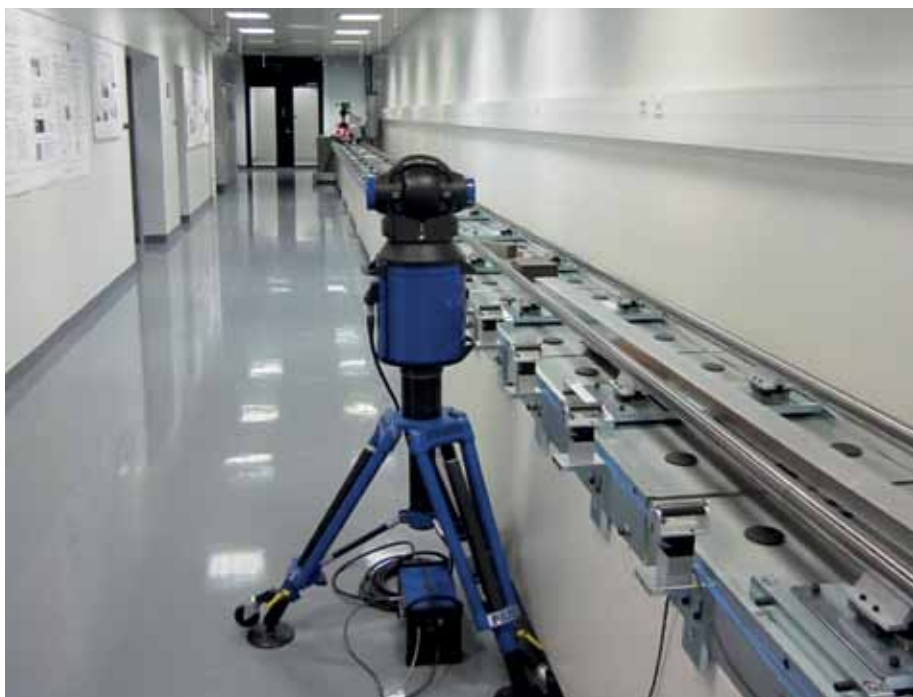
A laser tracker is calibrated against the MIKES 30-m interferometric bench.
