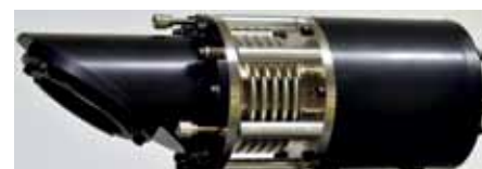
The room temperature PQED showing (from left to right) the Brewster window, adjustment screws, flexible bellows and the photodiode chamber. The total length of the detector is 215 mm.
