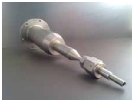
Measurement chamber with an entrance chamber of the first prototype for a calibration system for radiosondes designed at MIKES.
